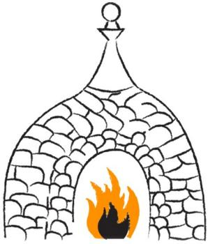
A *trullo* (plural, *trulli*) is a traditional, Apulian dry stone hut with a conical roof. Their style of construction is specific to the Italian region of Apulia. They are traditionally made with pure stone, without cement or mortar.
